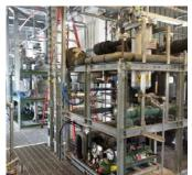
**Bath Cooler** Type of plant (Frigosolver©) Pieces 1 Nm³/h Flow rate 60 Condensation temperature °C 40 Cooling capacity kW 8 Operation pressure atm
