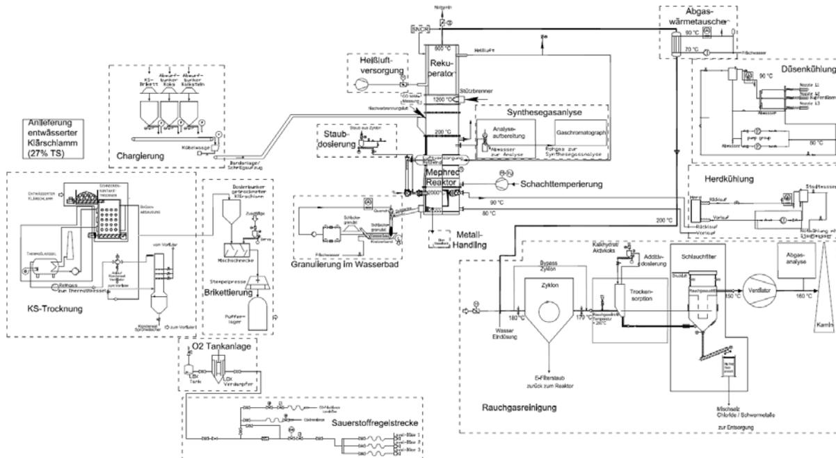
Figure 5: Flow diagram of pilot plant
