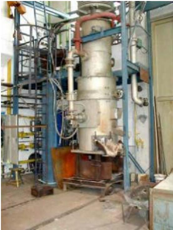
Figure 3: Small cupola furnace: Charging unit, circuit gas pipe, injector and drainage channel, furnace parameter [4]
