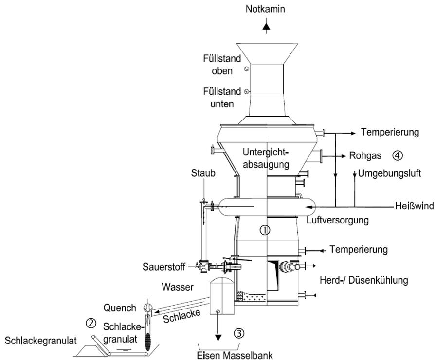
Figure 2: Schematic diagram of Mephrec®-reactor
